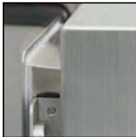
A special designed flat surface integral drainage channel prevents liquids or other solids contaminants from running in or falling into the enclosure when the door is opened. This design also prevent gasket from becoming broken when the door is tight closed.
