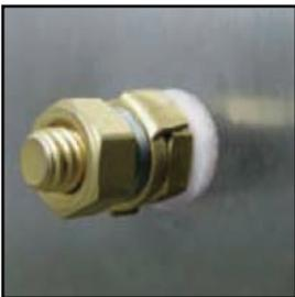
An integral external & internal feed through brass earth/ground stud assembly enables rapid and reliable protective earth/ground connection, mounted on the side of the enclosure, for ease of access.(Stainless steel earth/ground stud assembly as an option)
